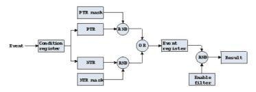
A group of registers starts with a **Condition register**. An internal **Event** will set the corresponding bit of the Condition register (to 'set a bit' means a transition from binary **0** to a binary **1**). Any Condition register will be updated continuously. This means that a bit will be reset as soon as the condition which rose that bit is no longer valid.
